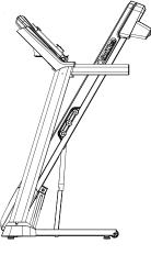
7. Make sure that the locking mechanism is engaged. Carefully pull back on the Walking Deck and make sure that it does not move. When you do this, keep clear of movement path in case the treadmill lock is not engaged.
