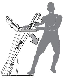
9. Grasping the Side Handrail and the front of the Upright, safely roll the treadmill to the desired location.
