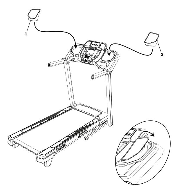
8. Attach the Base Shrouds to the Frame Assembly
